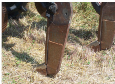
Straight subsoiler shanks without sweeps can work down to a 70 cm depth.
