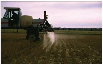
Low-drift nozzles (TD11004) operating at 60 psi
