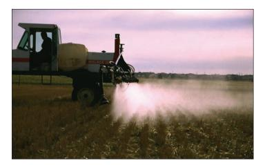
Conventional flat fan nozzles (XR8004) operating at 40 psi
