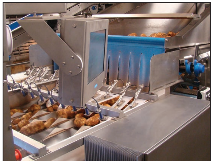
Potatoes run over the new optical grading equipment at Roll Bay Holdings.
