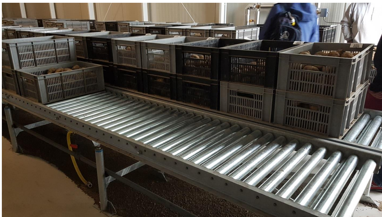
All samples from research plots in these trays on rollers to minimize labour.
