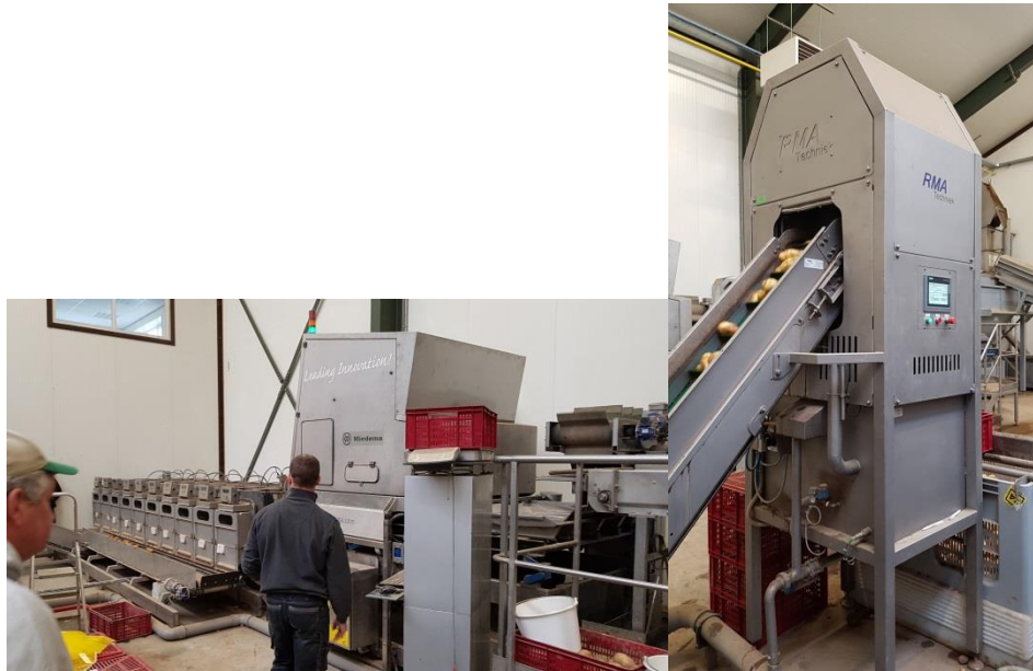
Automatic grading equipment at HZPC, including ability to do specific gravity.
