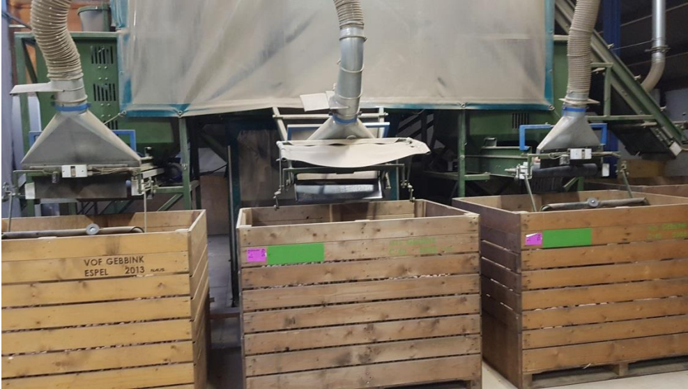
Sorting seed into 5 size categories with dust exhaust systems over each box.
