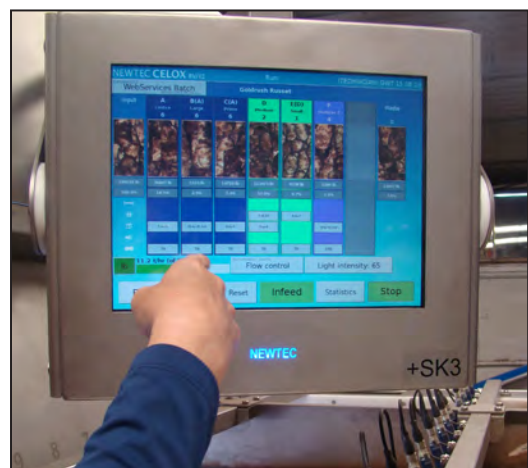
New optical grading equipment (above and previous page) installed at Rollo Bay Holdings near Souris allows the user to program the exact parameters for the grading line.
