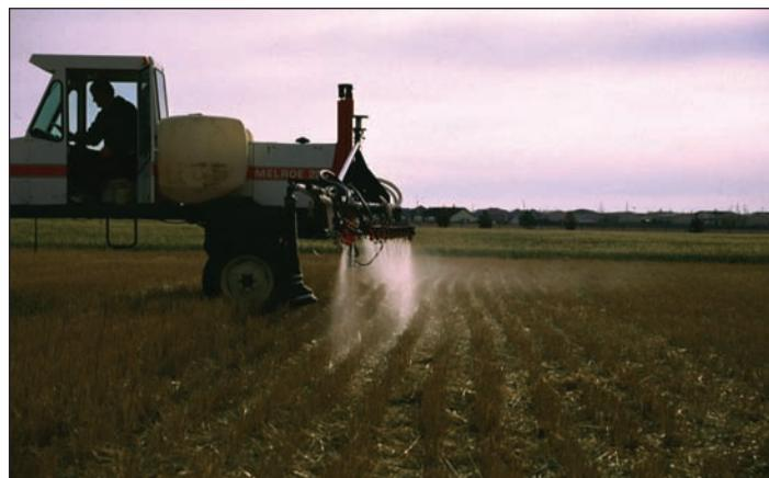
*Low-drift nozzles (TD11004) operating at 60 psi*
