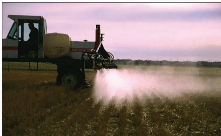
*Conventional flat fan nozzles (XR8004) operating at 40 psi*
