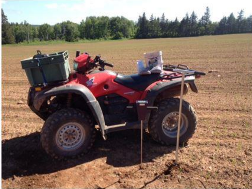
Figure 3: Tools used for collection of soil samples and compaction testing – PEI Potato Yield Variability Study 2016-1017
