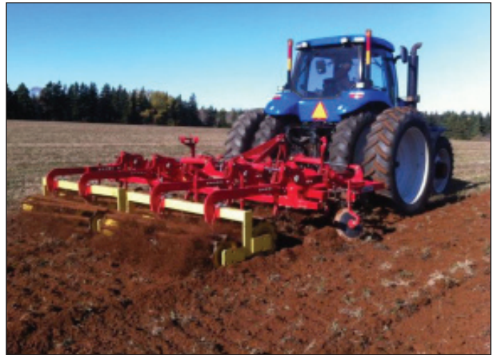
Pottinger Synkro 4003 tilling land in PEI. Photo: Tyler Wright.
