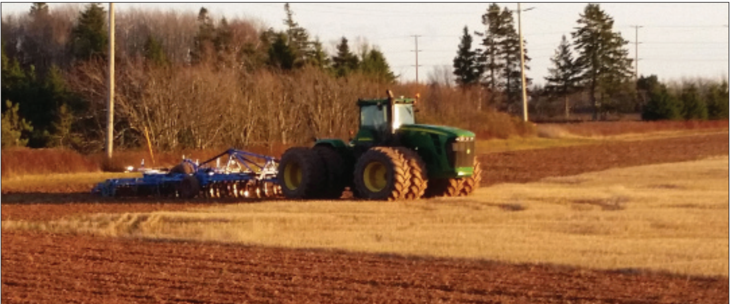
Lemken primary residue tillage (PRT) implement in use in Prince Edward Island. Photo: Mary Kay Sonier.
