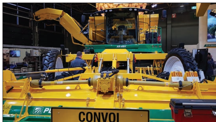
Ploeger 4 row self-propelled harvester with 14 tonne holding capacity. There are versions of this harvester now in North America.
