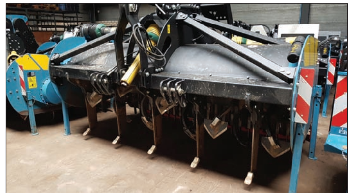
Imants "spader" tillage implement for land preparation in advance of potato production or for incorporation of biofumigant crops.
