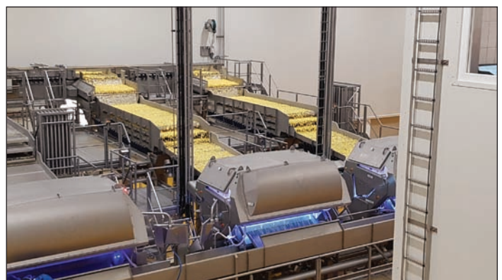
French fries coming off the cutters at the Agristo plant, headed for optical sorters to divert those requiring additional trimming.
