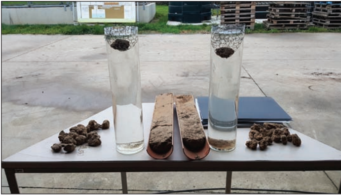
Demonstration of aggregate stability of soil at Bayer Forward Farm. Soil on left from min-till field, soil on right from moldboard ploughing.
