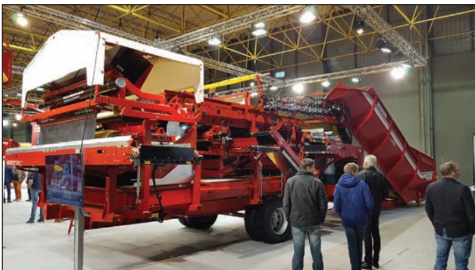
Large Grimme system for potato receiving, dirt elimination, optical sorting of dirt clods/rocks, and sizing of potatoes into multiple size groups.
