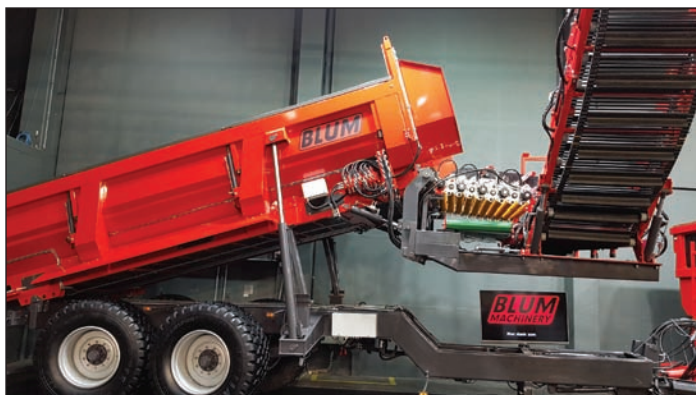
Crop wagon with dirt elimination and unloading elevator for transloading potatoes in the field. Trucks are not commonly used in the field in Belgium.
