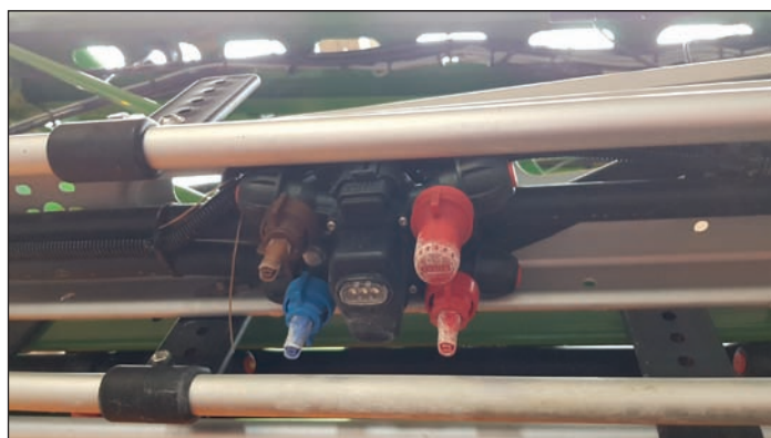
Multiple nozzle assembly on Amazone sprayer at ILVO. Each nozzle can be controlled individually across the entire sprayer for variable rate application.
