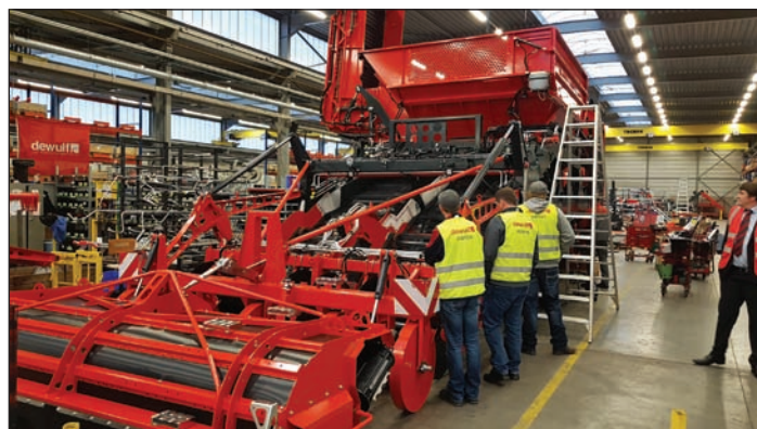
Dewulf self-propeller potato harvester under construction at the Dewulf factory in Roeselare, Belgium.
