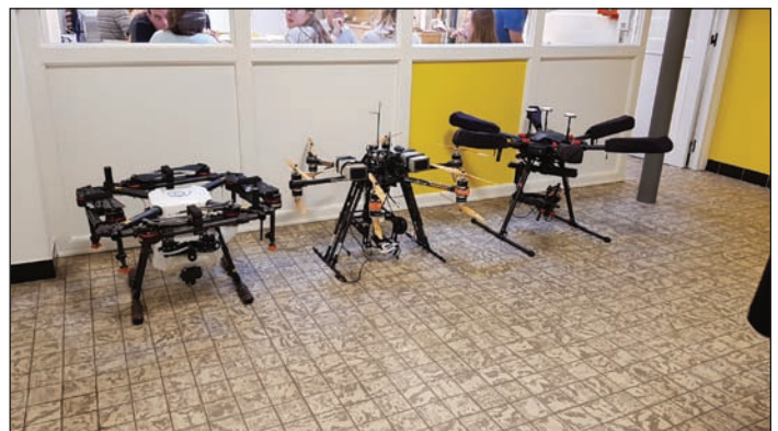
Drones under evaluation at ILVO near Ghent, including a drone (left) with a 12 litre tank for direct pesticide application.
