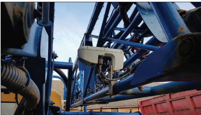
Sprayer mounted NDVI sensors for measurement of crop canopy biomass and N-response at Bayer Forward Farm.
