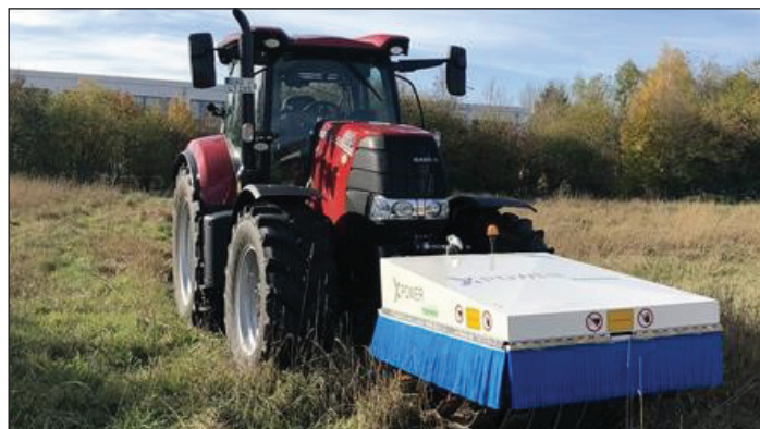
X-Power "electric herbicide" implement, a collaboration between Case New Holland and Zasso of Switzerland.
