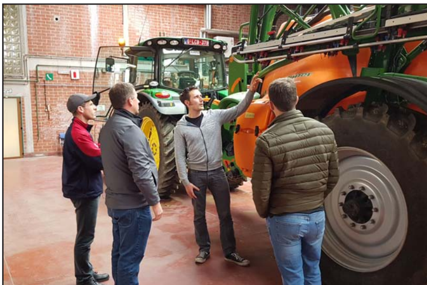
Dr. Simon Cool, (centre facing) of ILVO, explains some of the features for individual nozzle control on a potato sprayer that is used for variable rate spraying. Photo: R. Barrett.
