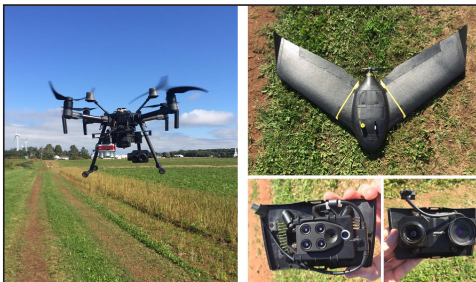
Figure 1: Pictured on the left is a multi-rotor DJI M210 that has two units onboard: a multispectral unit and a combined visual-thermal unit. Pictured on the top right is a fixed-wing senseFlyeBee X, which can only carry one unit at a time but offers a longer flight time. Pictured on the bottom right are a multispectral unit and a combined visual-thermal unit. (Photo credit: UPEI Climate Research Lab)
