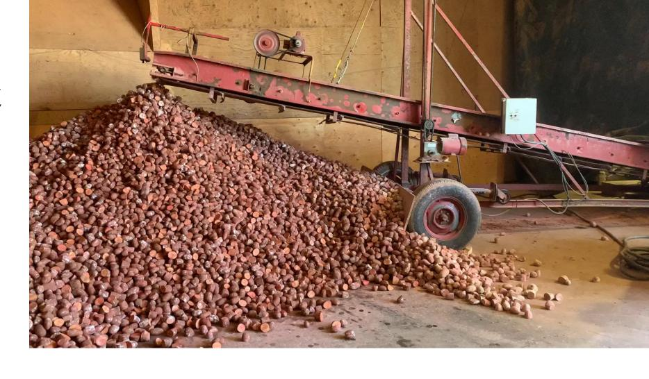
Optical Eye retrofitted to old bin piler to automatically adjust height
