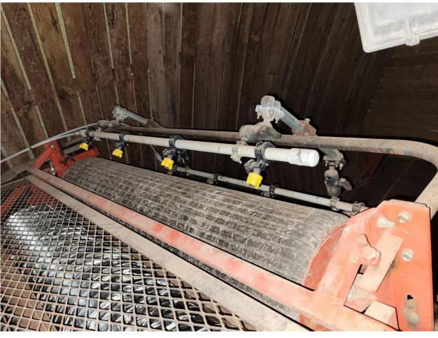
3 small booms with flat fan nozzles Spray for 10 seconds every 4 minutes when cutter was running
