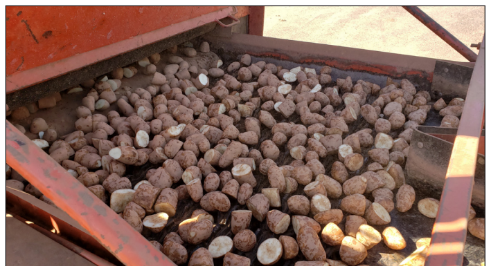
A consistent run of seed exiting the cutter. Chips and slivers have been removed, cut surfaces are clean, and seed piece size is consistent.
