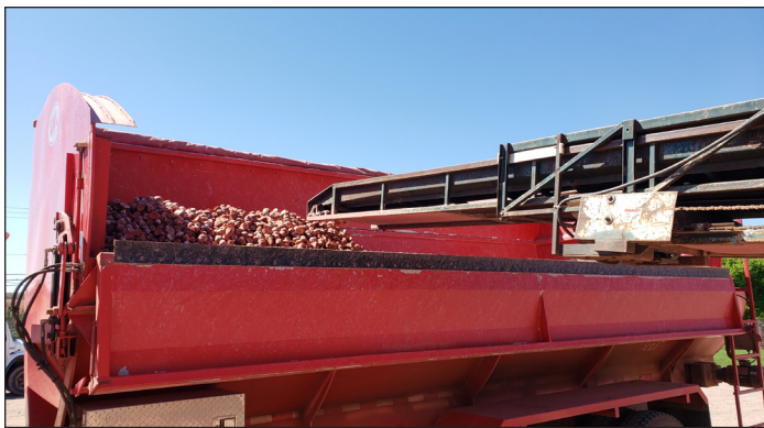
An example of loading seed with minimum drop height from the bin piler.
