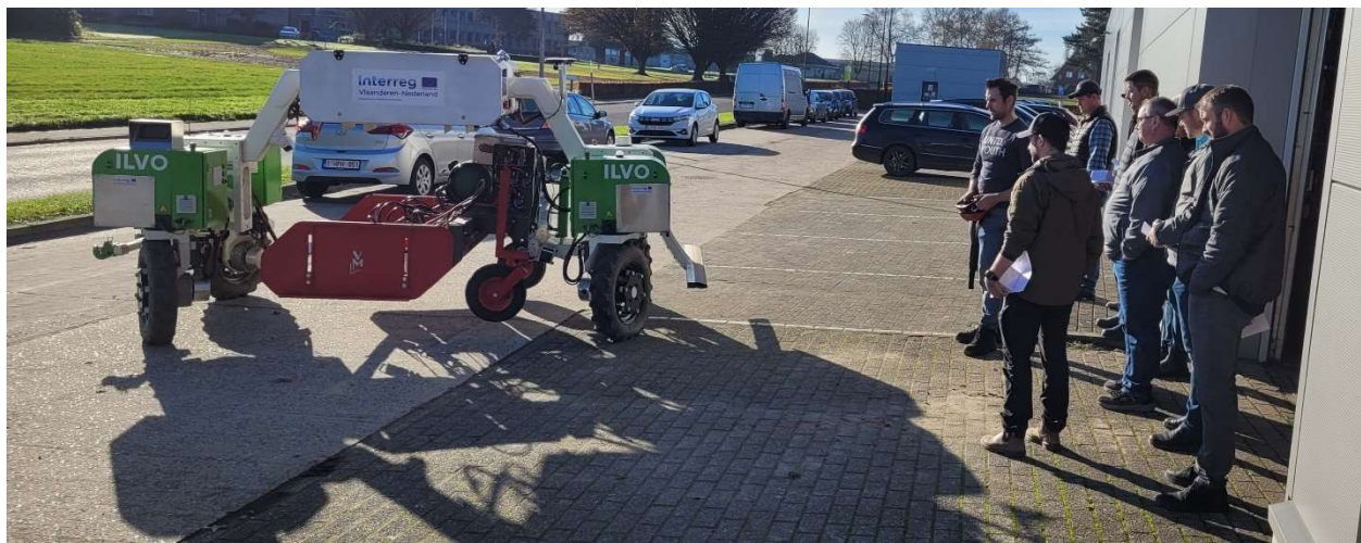
Robotic field vehicle at ILVO that can multiple attachments for field operations
