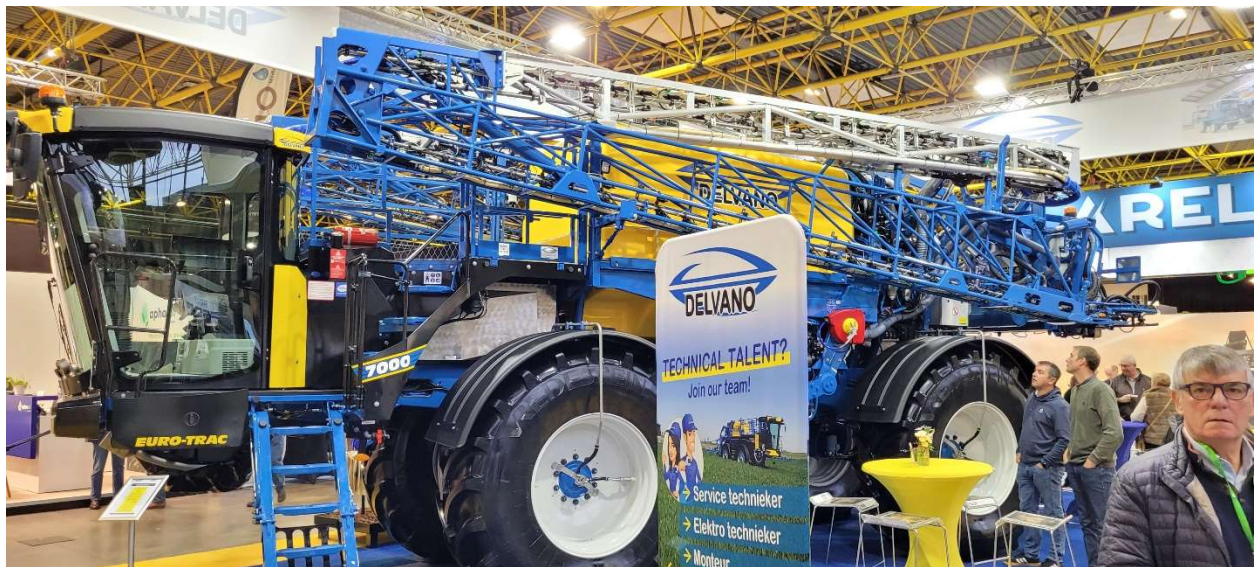
Delvano sprayer – Belgian company with up to 51 m boom width
