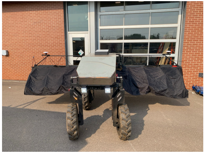
Figure 1. Foldable curtain design for easy transportation
