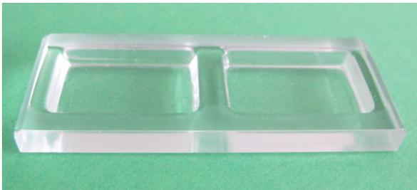
**Fig. 6** Counting chamber (courtesy Main Inspectorate of Plant Health and Seed Inspection - Central Laboratory, PL). (Note: the counting chambers shown here are specifically manufactured for the Main Inspectorate of Plant Health and Seed Inspection - Central Laboratory. Nematode counting chambers are also appropriate.) [Colour figure can be viewed at [wileyonlinelibrary.com](http://wileyonlinelibrary.com)]
