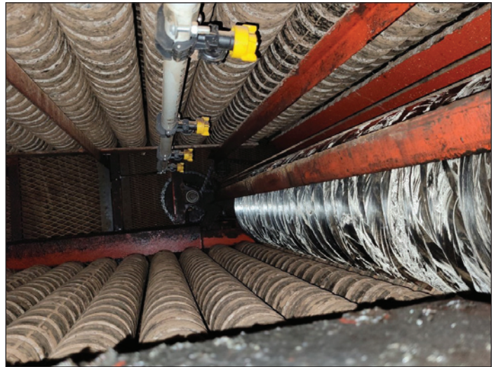
An example of a disinfection sprayer system added to a seed cutter, mounted directly ahead of the knives for periodic disinfection (every 10-15 min).
